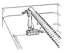
**To determine if the burner flame is proper,** light the burner. The flame should have 1/2" to 3/4" blue cones with no yellow tipping, and should not extend out over the baffle edges.
